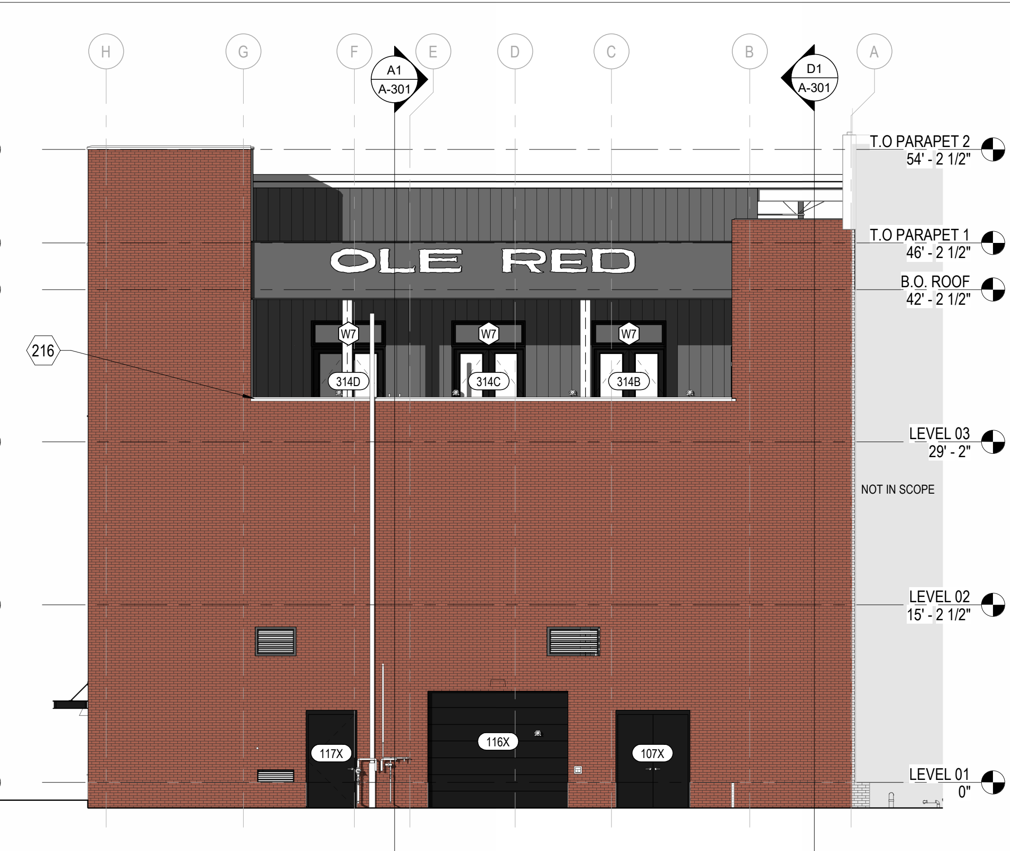
D4 EXTERIOR ELEVATION - EAST 1/8" = 1'-0"
