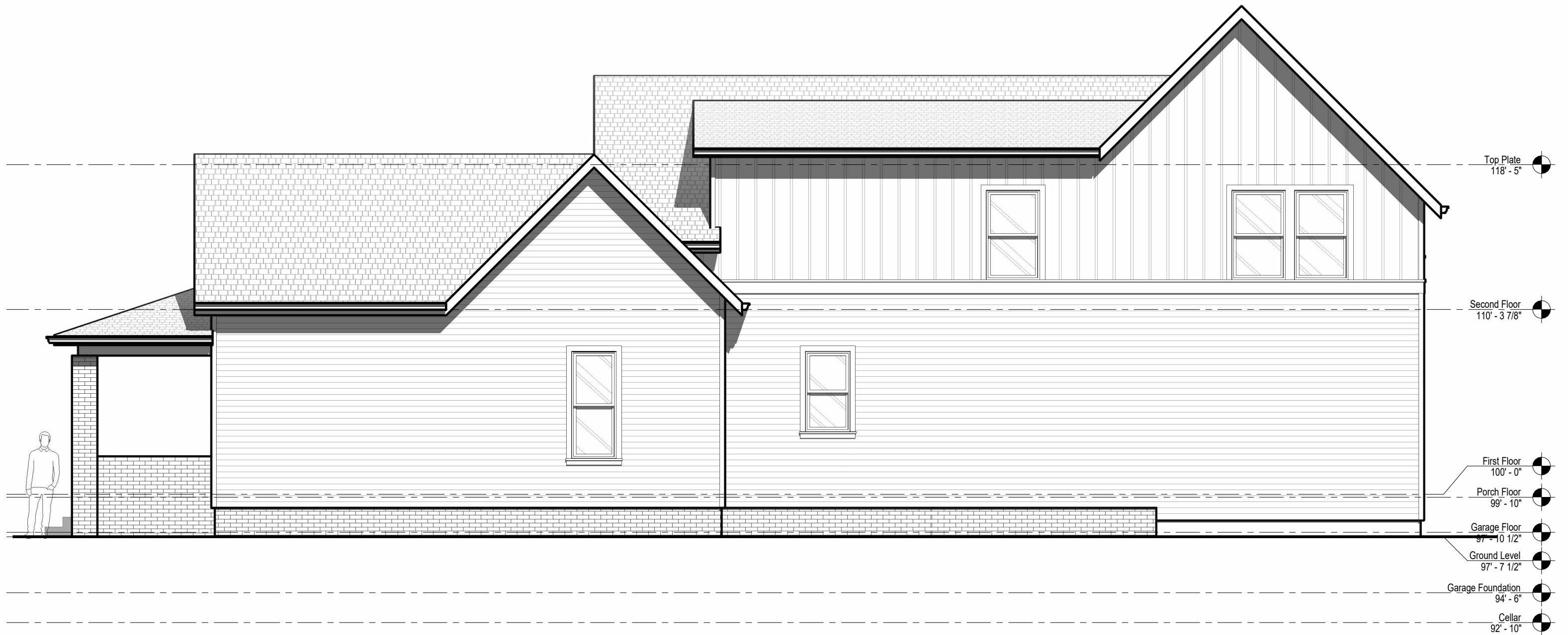
Building Elevation 1 East 3/16" = 1'-0"
