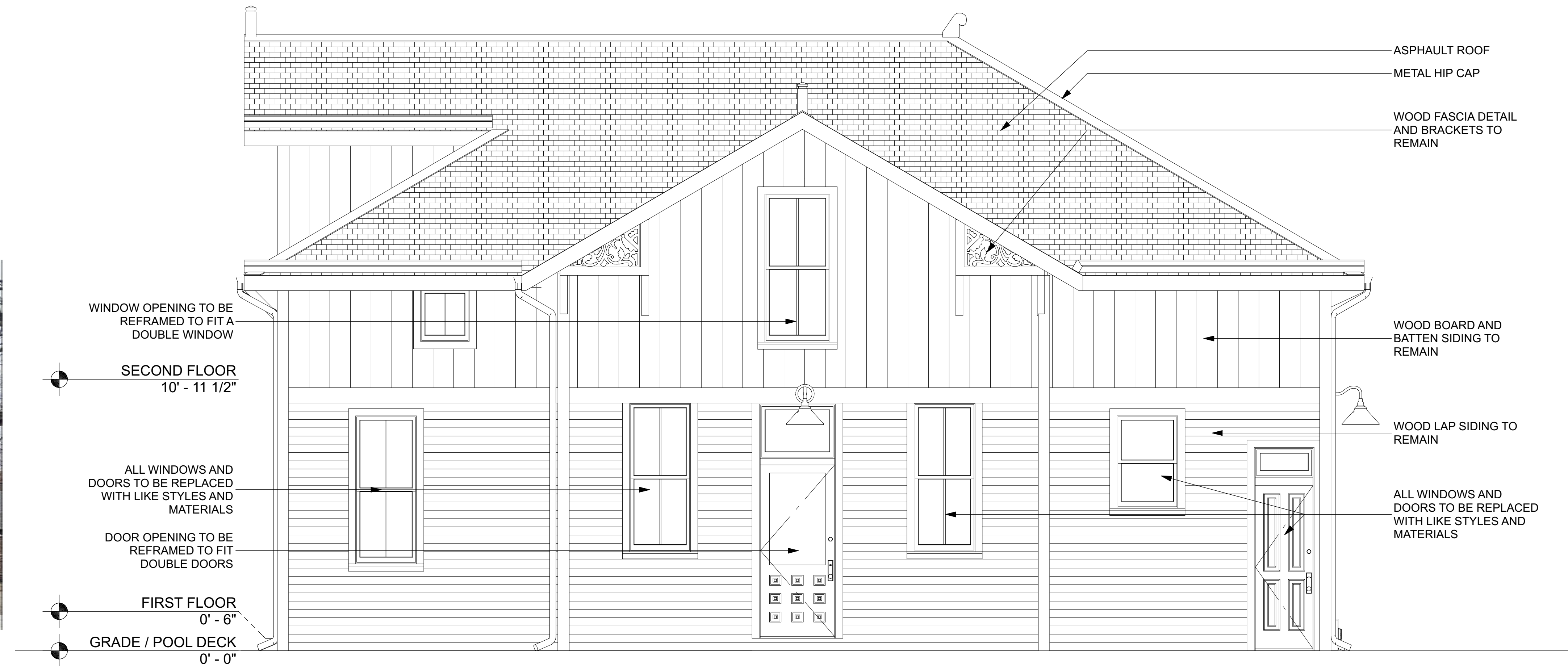
E5 EAST ELEVATION - PROPOSED 3/8 in = 1 ft ASPHALT ROOF METAL HIP CAP WINDOW SIZE TO REMAIN, WINDOW OPENING TO MOVE AND BE CENTERED ON GARAGE DOOR. SECOND MATCHING WINDOW GETS ADDED SECOND FLOOR 10' - 11 1/2" WOOD FASCIA DETAIL AND BRACKETS TO REMAIN WOOD BOARD AND BATTEN SIDING TO REMAIN WOOD LAP SIDING TO REMAIN GARAGE DOOR OPENING TO BE MOVED TO ACCOMODATE SECOND MATCHING GARAGE DOOR BEING ADDED FIRST FLOOR 0' - 6" GRADE / POOL DECK 0' - 0"
