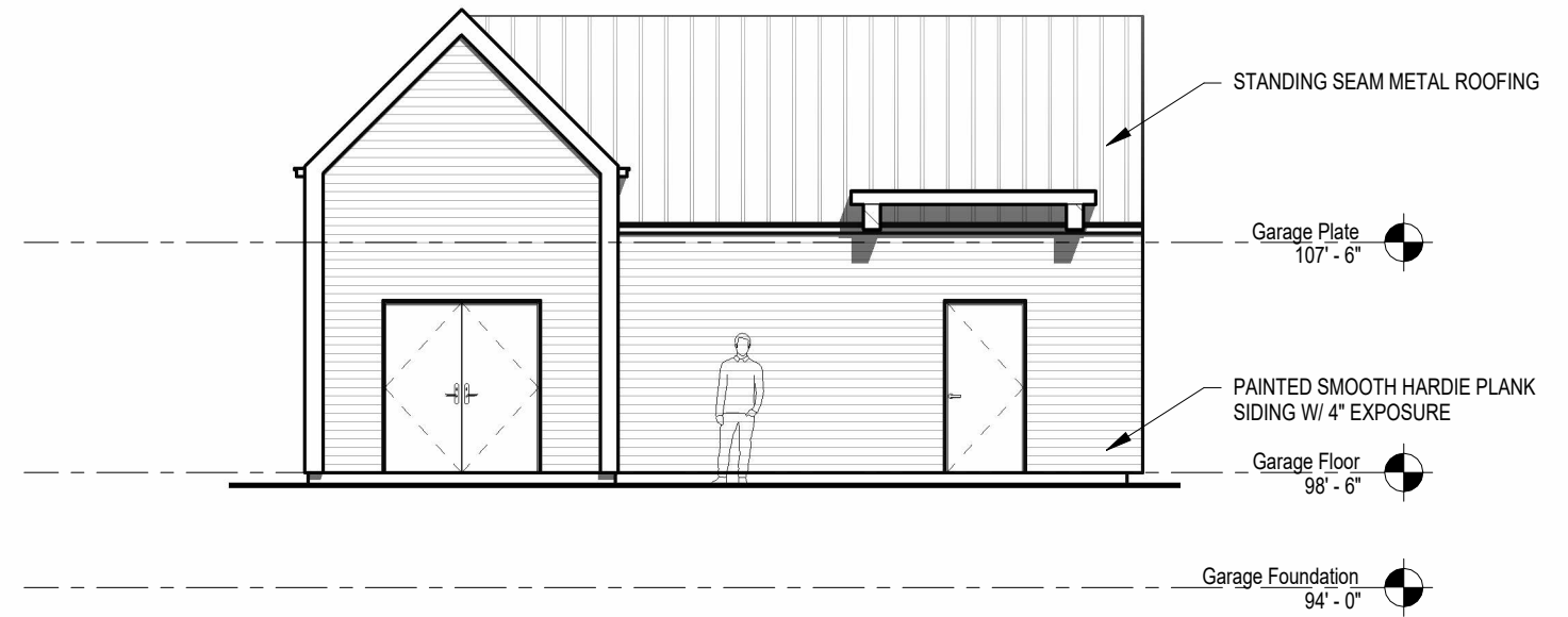
Building Elevation 1 Garage East 1/8" = 1'-0"
