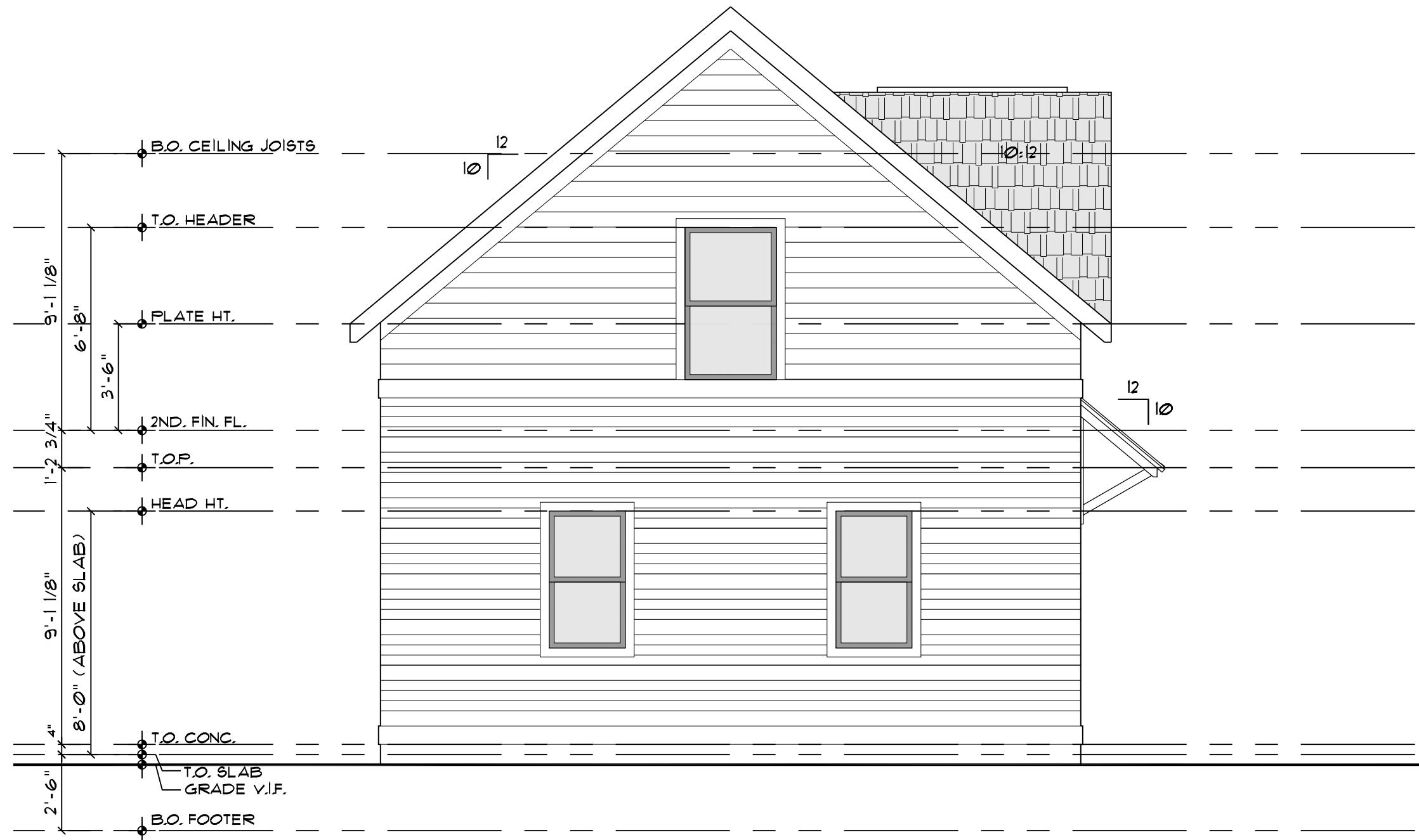
4 2133 N TALBOTT STREET GARAGE NORTH ELEVATION SCALE: 1/4" = 1'-0"
