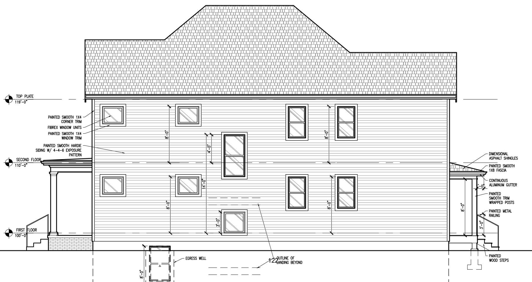
4 North Exterior Elevation 1/8"=1'-0" 0 4' 8' 16'
