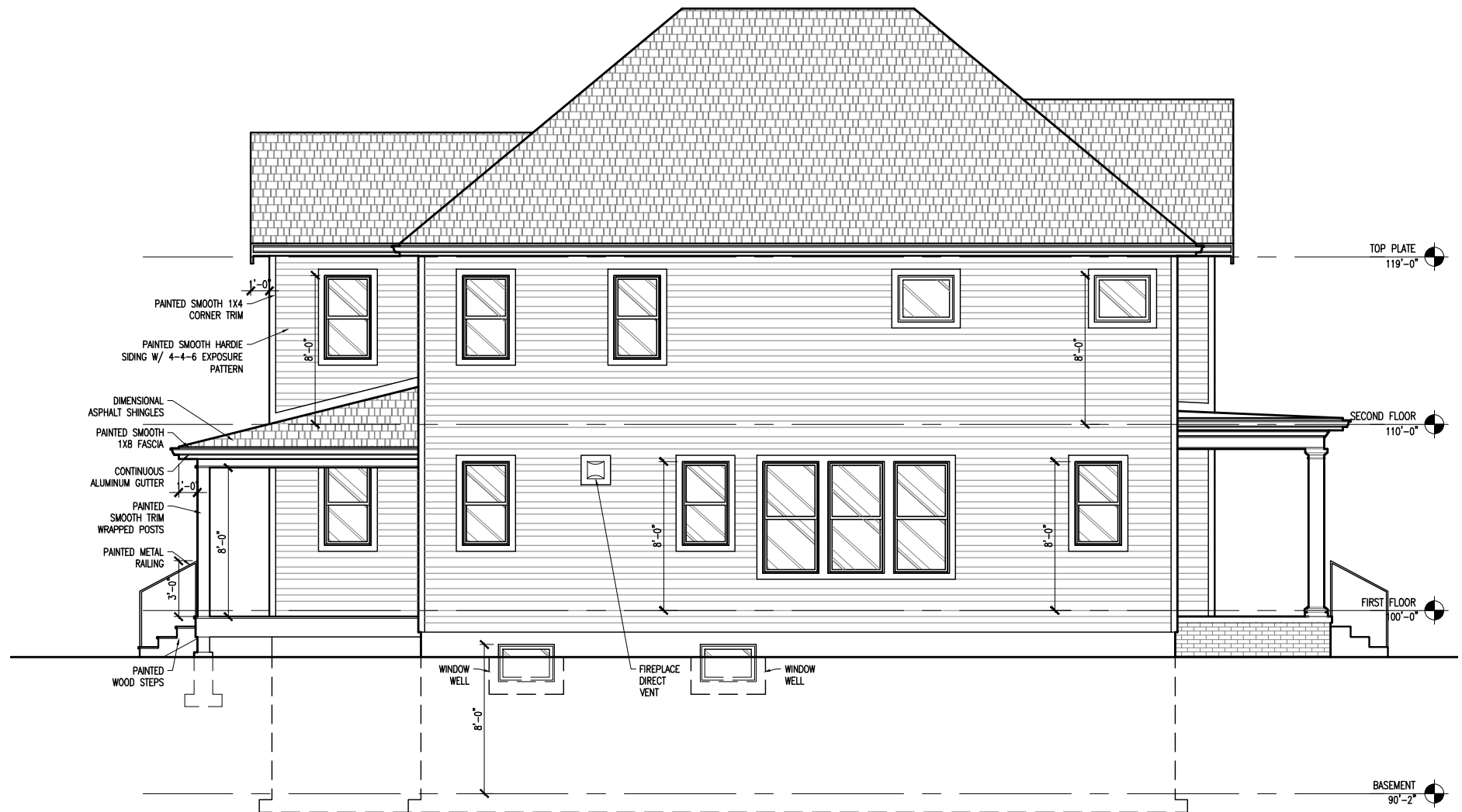
2 South Exterior Elevation 1/8"=1'-0" 0 4' 8' 16'
